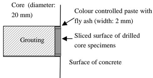
Figure 3 : Schematic description of repair of drilled hole
