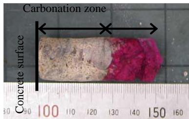
Photograph 3 : Carbonation of specimens
