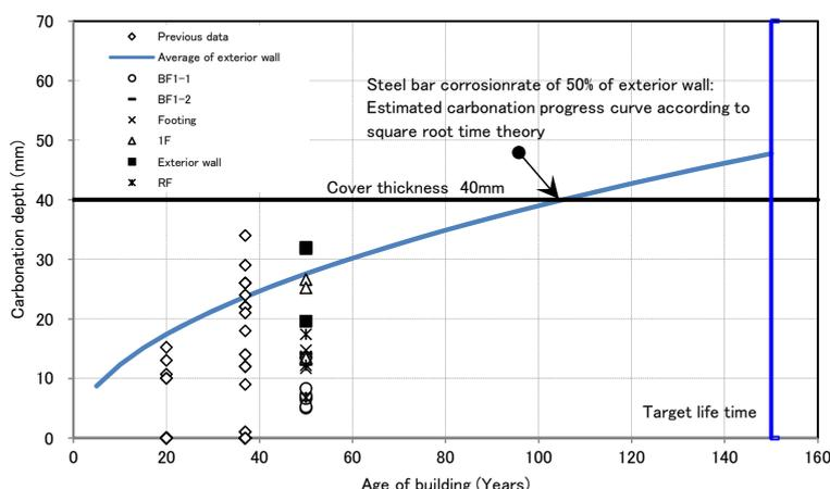
Figure 4: Carbonation progress of concrete by small core sampling test
