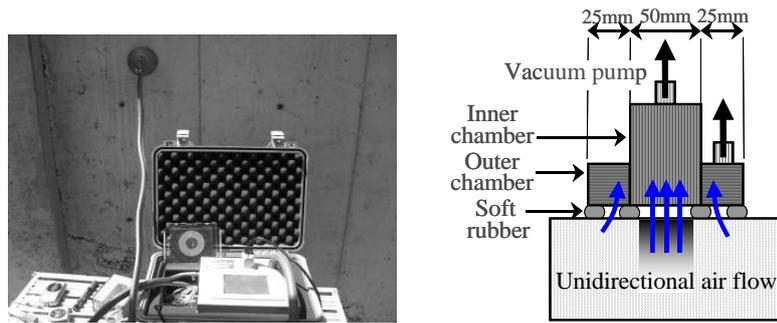
Figure: 2 Schematic description of Torrent permeability tester
