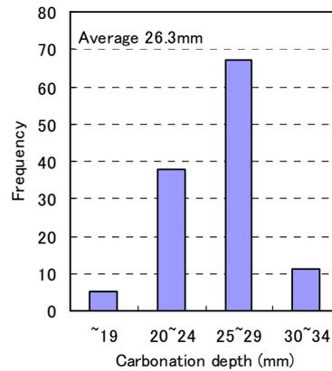
Figure 7: Distribution of carbonation depth
