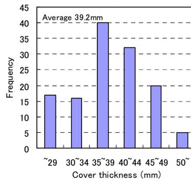
Figure 8: Distribution of cover thickness
