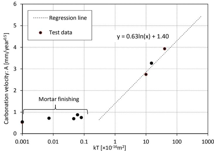
Figure 5: Relationship between carbonation and air permeability
